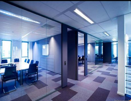
Interlight is a glazed partition system consisting of glazed panels from floor to ceiling, without any horizontal or vertical profiles. The glazed panels are assembled with a unique design which gives a seamless stable and modern appearance. The possibilities in glazing are almost unlimited, from standard to polarised glass, which can be transparent or opaque.
